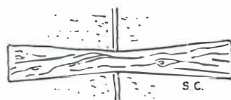
Fig. 123. Dovetail and wooden cramp, nearly five feet in length, in an architrave in the Court of Sheshonq at Karnak.
