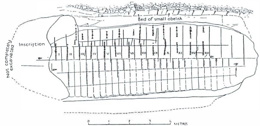
Fig. 29. Workmen's markings on the quarry-face near the Aswân obelisk.
