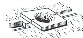
Fig. 202. Ventilation opening between two roof-slabs. Temple of Seti I at Abydos.
