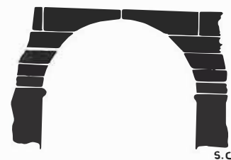
Fig. 221. Corbelled arch in the central sanctuary of the XVIIIth dynasty temple at El-Deir el-Bahari.
