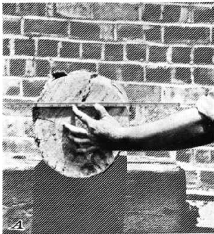
Compression wood in the outer annual layer of a southern pine: A , Extent of the compression wood formed in the circumference is indicated by the arc above the ruler; B , characteristic shelling of the outer layer of the wood due to excessive longitudinal shrinkage of the compression wood.
