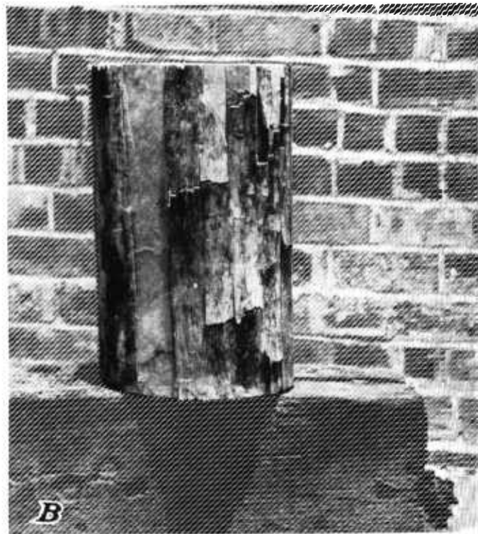
Compression wood in the outer annual layer of a southern pine: A , Extent of the compression wood formed in the circumference is indicated by the arc above the ruler; B , characteristic shelling of the outer layer of the wood due to excessive longitudinal shrinkage of the compression wood.
